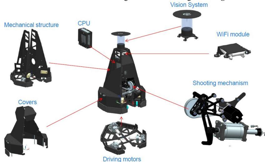
The supporting frame of the robot consists of 6mm thick steel. Sheet metal parts are used to reduce costs and milling time. The covers of the robot are made of 3mm aluminum sheets. The Turtle 5k uses 3 separate motors that drive 3 omni-wheels which allow the robot to move freely in any direction.
