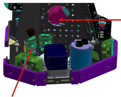
New smart motor i.s.o. heavy stepper motor and stepper motor driverd
