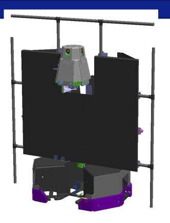
Carbon fiber tubes on stainless steel frame with 3 home made solenoids
